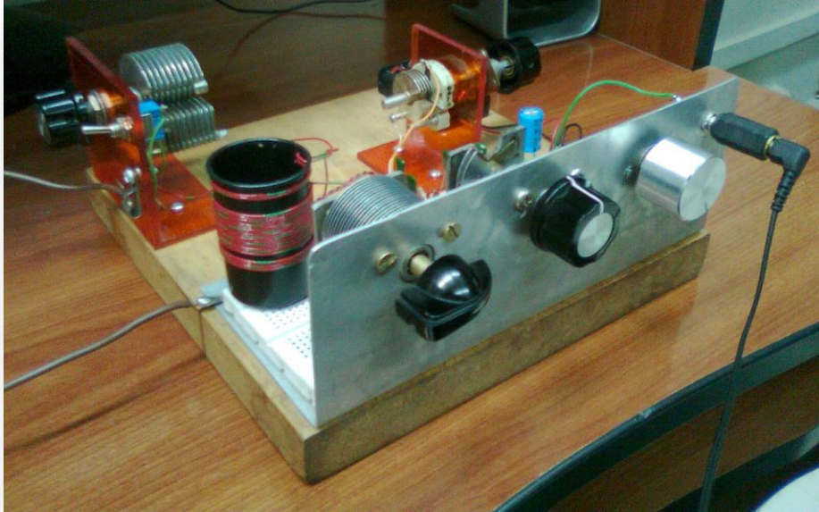
Fig.3.a Front panel with main tuning capacitor, bandspread capacitor and volume control
