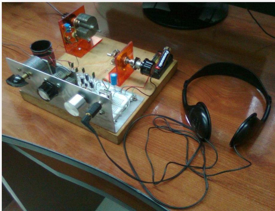
Fig.3.a Front panel with main tuning capacitor, bandspread capacitor and volume control
